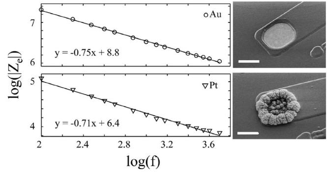
Fig. 3. The average impedance magnitudes and linear fits for gold ( $n = 12$ ,  $r^2 = 0.947$ ) and platinized microelectrodes ( $n = 9$ ,  $r^2 = 0.870$ ) as a function of frequency (0.1–5 kHz). Images on the right are SEM micrographs of a gold recording site and a platinized site. Scale bars = 5  $\mu\text{m}$ .
