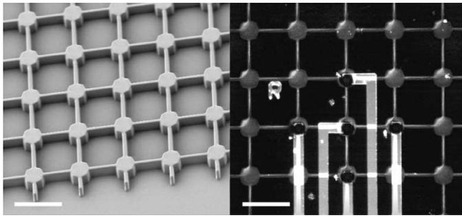
Fig. 4. (a) SEM micrograph of a PDMS stamp. (b) Pattern of FITC-labeled PLL produced by aligning the stamp's features to the recording sites. Scale bars = 50  $\mu\text{m}$ .
