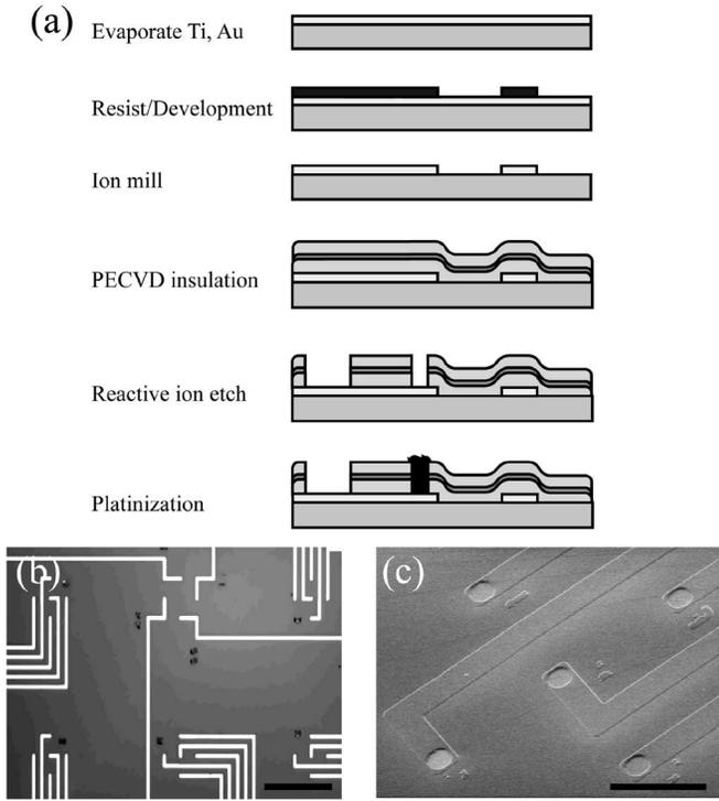
Fig. 1. (a) MEA fabrication process and (b) optical micrograph of six sets of microelectrodes on the device. Scale bar = 200  $\mu\text{m}$ . (c) SEM micrograph of a set of microelectrodes. Scale bar = 25  $\mu\text{m}$ .
